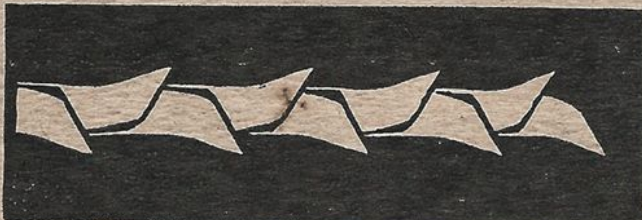
FIG. 6 Looking down on the tooth-edge (magnified) of a cross-cut saw properly set.
