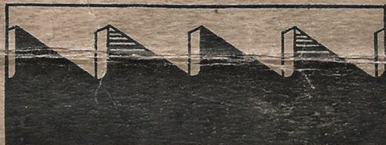
FIG. 2 Teeth of Rip Saw (Magnified) Showing correct shape.
