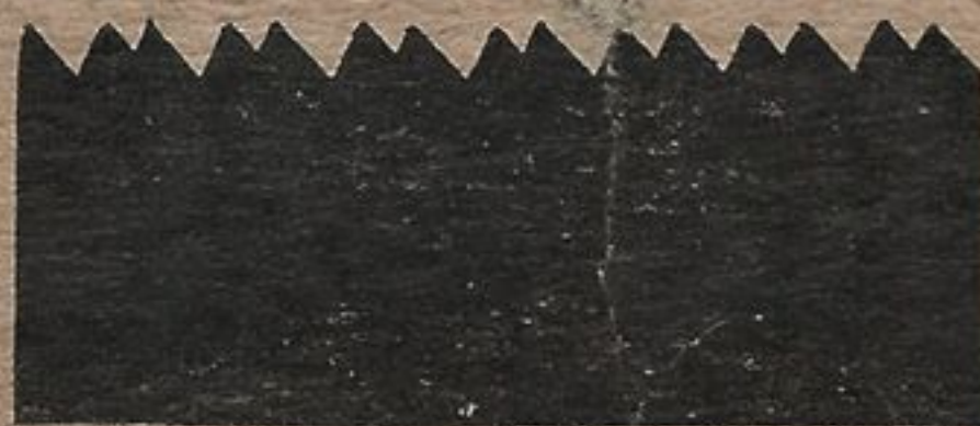
FIG. 4 This saw needs jointing. Read directions below.
