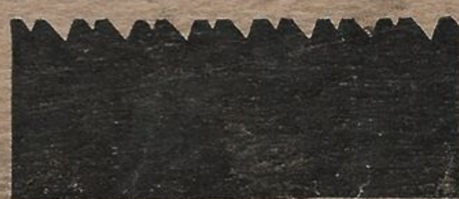
FIG. 5 The saw in Fig. 4 after jointing. "Shape the Teeth" next. Read directions below.
