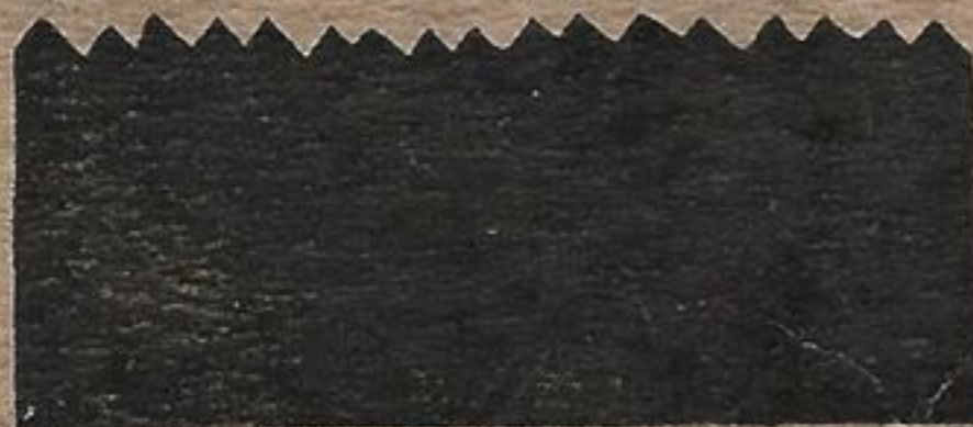
FIG. 3 If the teeth of your saw are so uneven as this, it probably needs to go back to the maker to be put into good condition.
